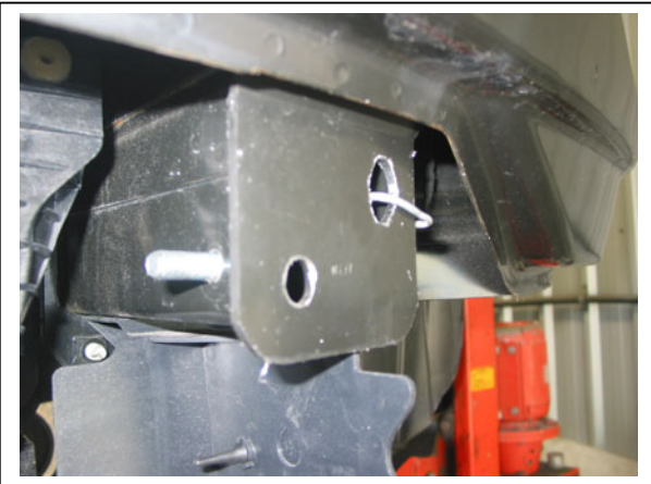
Figure 5: Cut and crimp wire to side of opening
